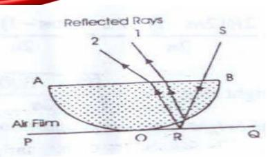
The thickness of air-film remains constant along a circle with its centre at O. Hence, the fringes are in the form of concentric circles.
