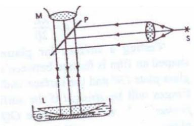
If monochromatic light is allowed to fall normally on this film, a system of alternate bright and dark concentric rings is formed in the air film.
